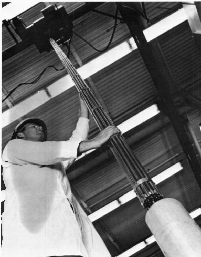
A technician inspects a prototype nuclear reactor fuel rod. This type of rod was manufactured at the Kerr-McGee Facility. Photo courtesy of U.S. Department of Energy.
