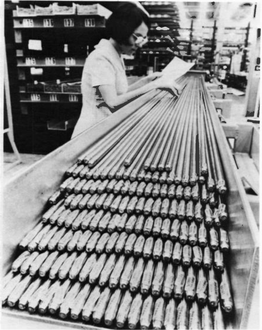
Completed nuclear fuel rods undergo a final visual inspection by an employee. With the aid of a computer, color and number coded labels at the end of each rod allow quality control personnel to trace the origin of zirconium in the rod. Each rod contains uranium dioxide fuel pellets and, in a nuclear power plant, can produce as much energy as more than 200 tons of coal. A Westinghouse photo by Jack Merhaut; courtesy of U.S. Department of Energy.
