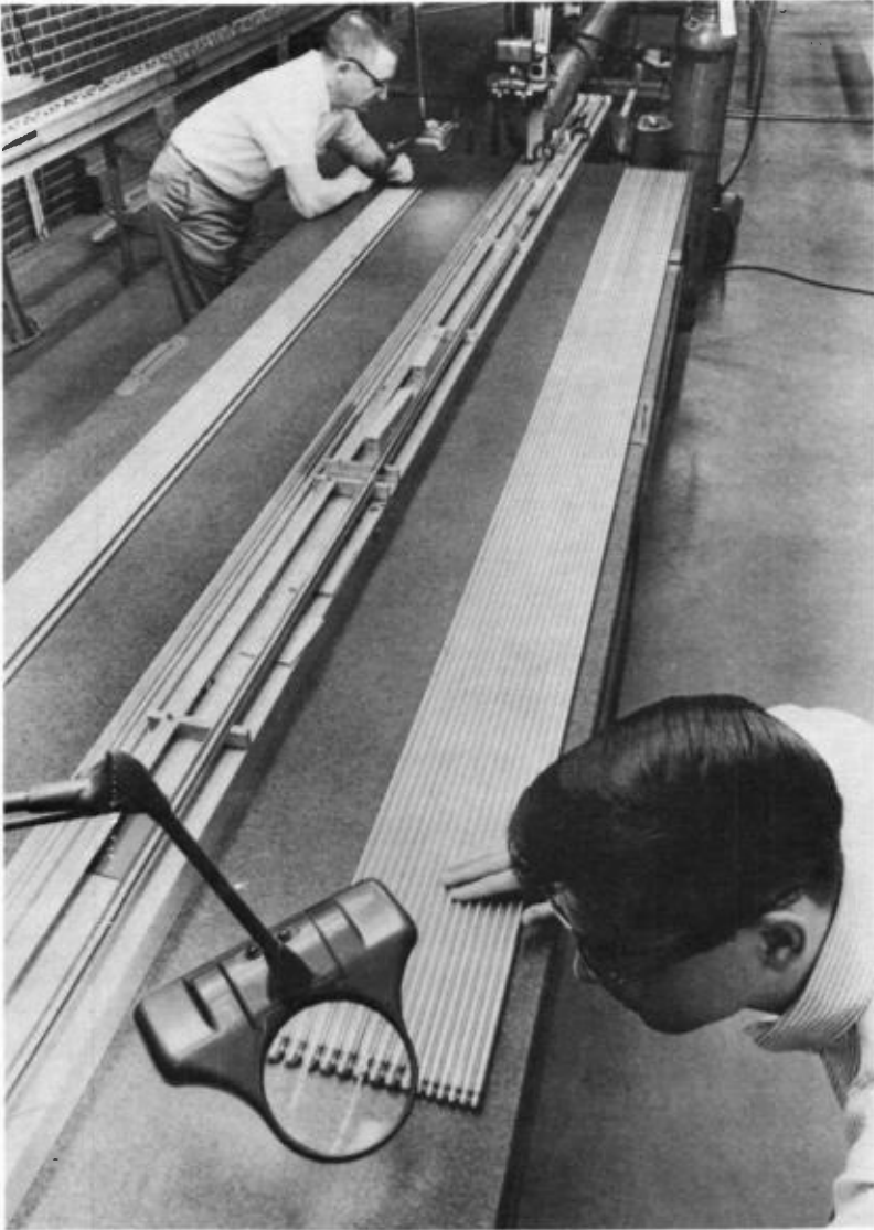
Inspectors check end-cap welds on zirconium alloy rods containing nuclear fuel pellets prior to installation of the rods in a fuel assembly. Each rod contains about 200 one-ounce pellets and can supply the energy needed to generate enough electricity to meet annual residential requirements of about 200 people. A Westinghouse photo; courtesy of U.S. Department of Energy.
